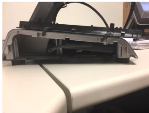
Figure 27 – HP RP9 Base Note, Large Power Brick in Base
